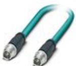
Network cable, Ethernet CAT6<sub>A</sub> (10 Gbps), CC-Link IE CAT6<sub>A</sub> (10 Gbps), 8-position, PUR halogen-free, water blue RAL 5021, shielded (Advanced Shielding Technology), Plug straight M12 / IP67, coding: X, on Plug straight M12 / IP67, coding: X, cable length: 1 m
