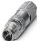
Data connector, Ethernet CAT6<sub>A</sub> (10 Gbps), 8-position, shielded, Plug straight M12 SPEEDCON, Coding: X, Piercecon<sup>®</sup>, knurl material: Zinc die-cast, nickel-plated, external cable diameter 4 mm ... 8 mm
