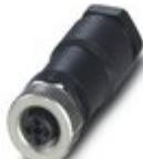
Power connector, Power, 4-position, unshielded, Socket straight M12, Coding: T, Screw connection, knurl material: Zinc die-cast, nickel-plated, cable gland Pg11, external cable diameter 8 mm ... 10 mm, For direct current up to 12 A/63 V
