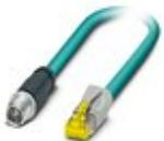
Network cable, Ethernet CAT6<sub>A</sub> (10 Gbps), CC-Link IE CAT6<sub>A</sub> (10 Gbps), 8-position, PUR halogen-free, water blue RAL 5021, shielded (Advanced Shielding Technology), Plug straight M12 / IP67, coding: X, on Plug straight RJ45 / IP20, cable length: 2 m
