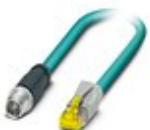
Network cable, Ethernet CAT6<sub>A</sub> (10 Gbps), CC-Link IE CAT6<sub>A</sub> (10 Gbps), 8-position, PUR halogen-free, water blue RAL 5021, shielded (Advanced Shielding Technology), Plug straight M12 / IP67, coding: X, on Plug straight RJ45 / IP20, coding: X, cable length: 1 m
